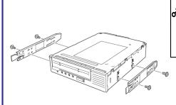
Please use the correct latching rails which are attached with the Use the screws attached to the Built-in LTO for latching rails. The attached screws are metric Screws (4.0 mm length, 3.5 mm under its washer).
