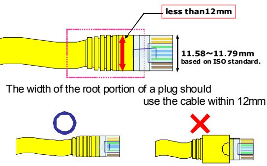
Refer to the left figure which does not get used to use for the cable with boots (with a connector cover).
