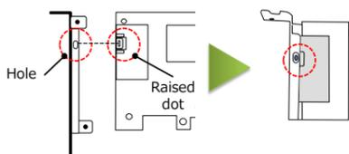
2. Rotate the bracket toward the arrow and attach it.
