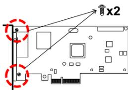
2. As shown in the figure on the left side of the figure below, Rotate the bracket toward the arrow and remove it.
