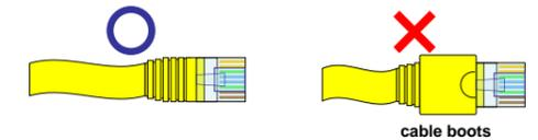
Refer to the left figure which does not get used to use for the cable with boots (with a connector cover).
