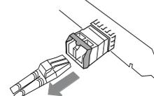
2. Flip down the Lever of the SFP+ module, then Remove the module from the slot toward to the arrow
