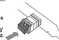
3. Remove the Dust Cover from this product, and Connect the Cable firmly.
