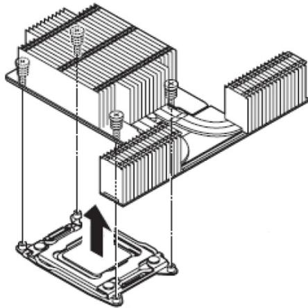
2. Install the Heat Sink of this Kit to CPU2.
