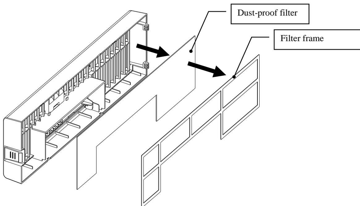
2.2 Replace of the dust-proof filter then insert the dust-proof filter and filter frame.
