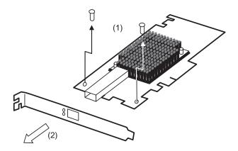
**3**. Install the low profile bracket to this product and tighten the two screws.
