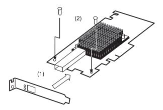
4. Replace the SFP+ module removed in item 1.
