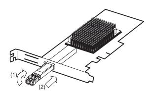
**6**. Replace the cover and components removed in item 2. (Take care not to conflict the SFP+ module with the cover edge.)
