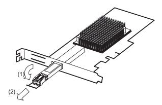
2. Remove the two screws and remove the bracket from this product.
