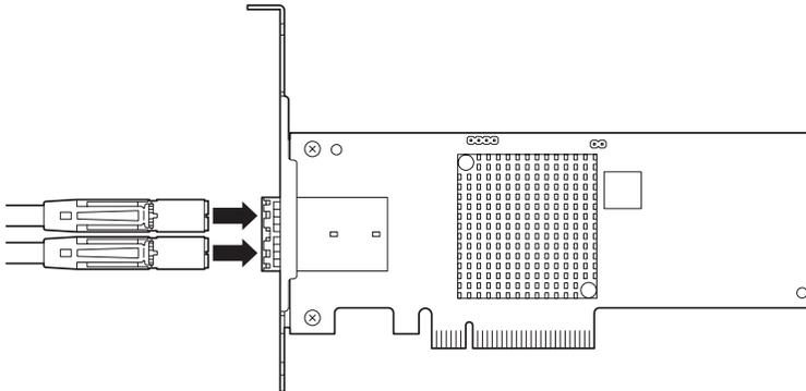
3. Insert a cable connector (the other side) in SAS device's connector fully for firm connection.
